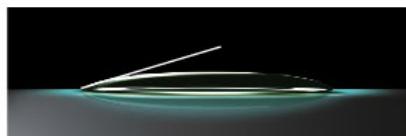
Identium® after 1 sec.: contact angle < 10°
